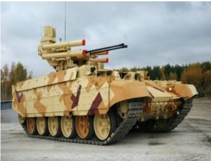
The BMPT "Terminator" is a post-Cold war armored fighting vehicle (AFV) designed for supporting tanks and other AFVs. It was designed to survive in urban combat and armed with four missile launchers, two 30 mm cannons, two grenade launchers and one coaxial 7.62 mm machine gun. The BMPT is built on the chassis of the T-72 main battle tank. Russia appears to have foregone procurement of the Terminator in favor of the T-15 IFV.
