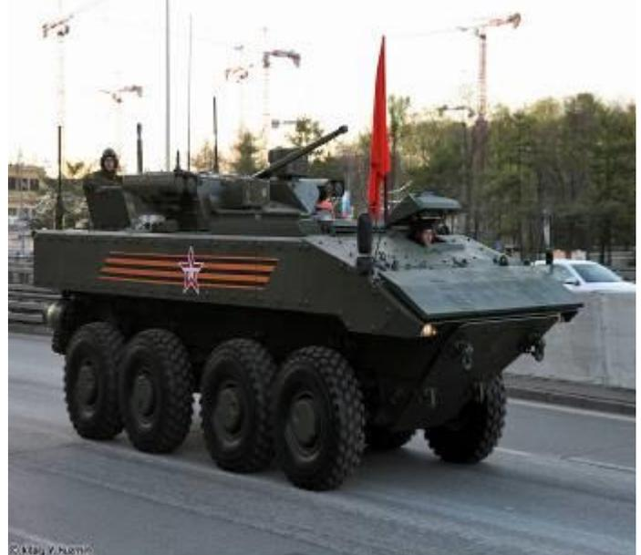
The Russian "Boomerang" is a modern 8x8 Wheeled amphibious vehicle designed to replace the BTR 60/70/80 series of wheeled personnel carriers. They can negotiate and overcome water obstacles and use two water jets. The engine is located in the front instead of the rear. Engine location was a significant drawback of BTR vehicles, where soldiers had to exit the vehicles through cramped side doors, which
