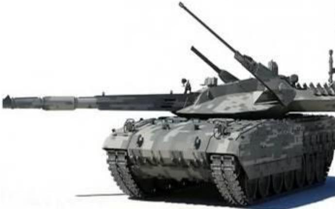
This image may be a better representation of what the final production version of the Armata may look like. It appears to have a 152mm main gun, a 30mm cannon on the left side of the turret and a 12.7 mm rotary gun on the right. It also has heavily sloped appliqué armor.
