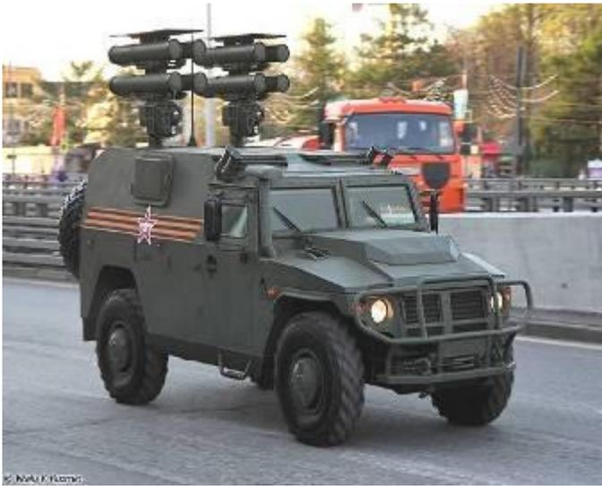
The GAZ Tiger is a Russian 4x4, multipurpose, all-terrain infantry mobility vehicle. It is similar in appearance and performance to the US HMMWV. The Tiger is versatile and can carry a large variety of weapons. The photo above shows the SPM-2 anti-tank version. It's equipped with two retractable launchers for 8 missiles and a remote weapons control system with screens that display images from the sighting systems. It carries eight additional missiles.
