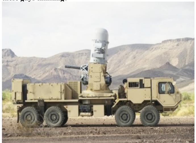
This interesting vehicle is an 8X8 HEMTT A3 mounting a 20mm Phalanx Close in Weapons System. They are used to protect military bases against incoming rocket and mortar rounds. They are quite effective and destroy the rounds by direct impact. They are not proximity fuses.
