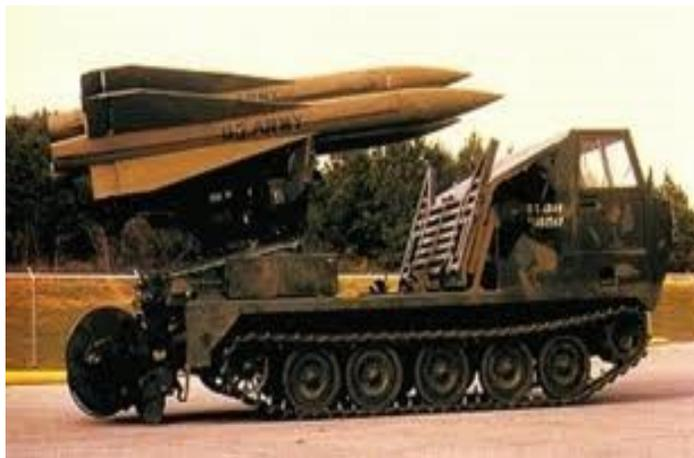
This is a photo of the M548 tracked launcher. It was a modified version of the M113 chassis that could transport and launch the Hawk missiles. It could carry the missiles for long distances and had a built-in launcher for quick deployment. They were only used for a short period of time and never fully adopted by the US Army.
