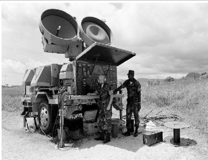
This is a photo of the combined Doppler illumination and targeting missile tracking radar.
