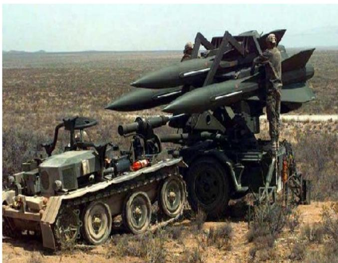
The XM501 E2 loader/transporter was designed used for loading missiles on the launcher and transporting them in and around the battery area.
