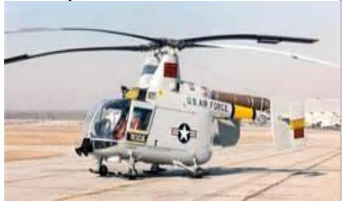
The main role of the Kaman HH-43 Huskies was rescue. They were usually restricted to working on airfields. It would use its rotor wash, and a foam spraying unit hanging on a sling, to hold back the flames while the firefighters tried to rescue crew from burning aircraft.
