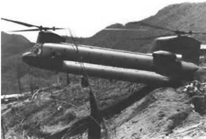
The CH-47 Chinook was used in a variety of roles. They could carry troops, cargo, and even small vehicles inside. They could also use a sling to carry cargo, vehicles, artillery pieces and to recover downed helicopters and aircraft.
