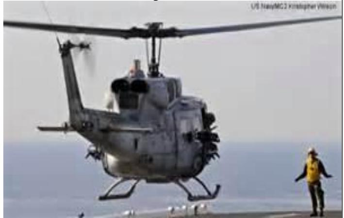
The UH-1E, F, L, N, and P were designations used for Air Force, Navy, and Marine Corp models. There were even twin engine versions called the Bell 212 in civilian service. By the end of the war, Bell had tripled the gross weight of the Huey without increasing the size of the fuselage.
